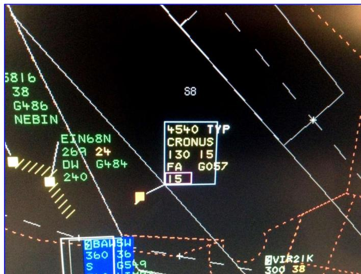
Figure 6-17: Limited Trail Dots on Controller's Display
